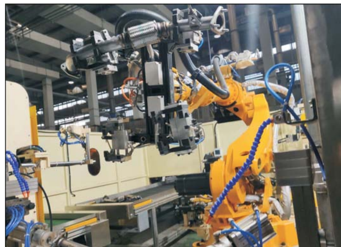
► Welding of automobile exhaust pipe
